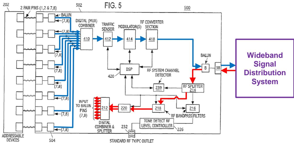
The exemplary system of Fig. 5 is capable of both sending RF signals to, and receiving RF signals from, a wideband signal distribution system via
