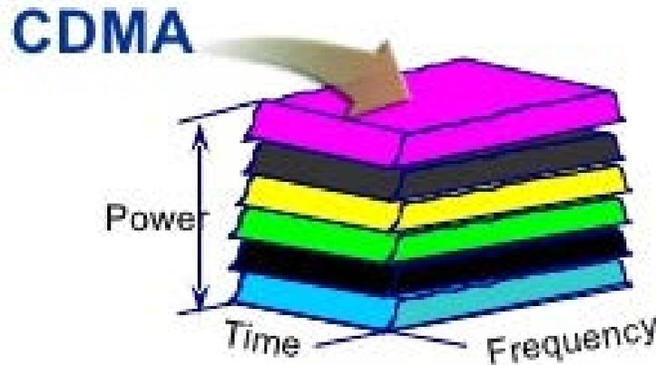
*Id.* As shown in the diagram, all data streams are simultaneously transmitted over *the same* RF channel.
