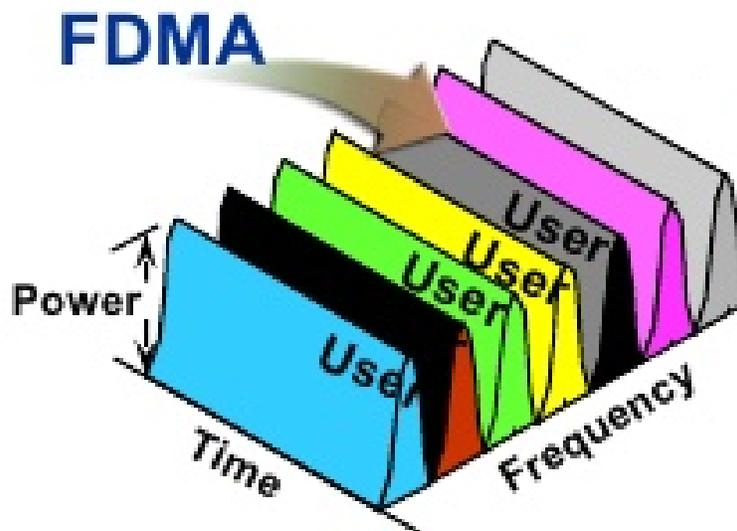
*Id.* As shown in the diagram, each data stream is assigned to an RF channel on a frequency band that does not change over time. As stated by Mr. Wechselberger, the "type of multiplexing discussed in the '679 patent[] involves dividing the RF
